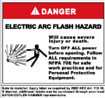
**Figure 1 - Minimum Required Labeling**
